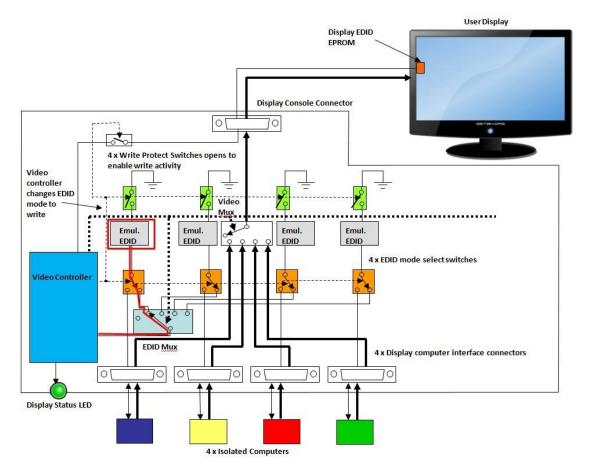
Figure 5 – Display EDID Write Function
